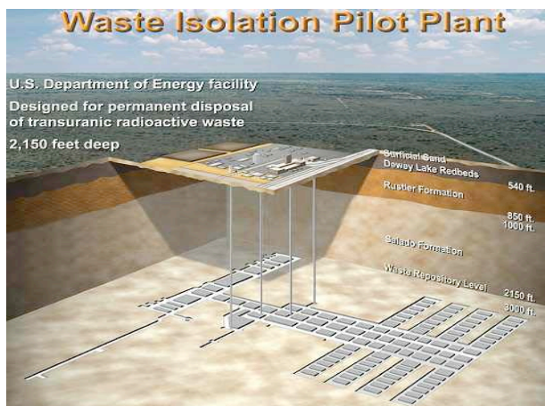
Fig. 4. The Waste Isolation Pilot Plant (WIPP), the only operating deep geologic nuclear waste repository, is excavated 700 meters below the surface in the massive salt of the Salado Formation, and has operating successfully since 1999.
