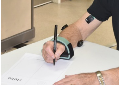
Figure 2. Sketch of the brace and sensors (EMGs) being worn.
