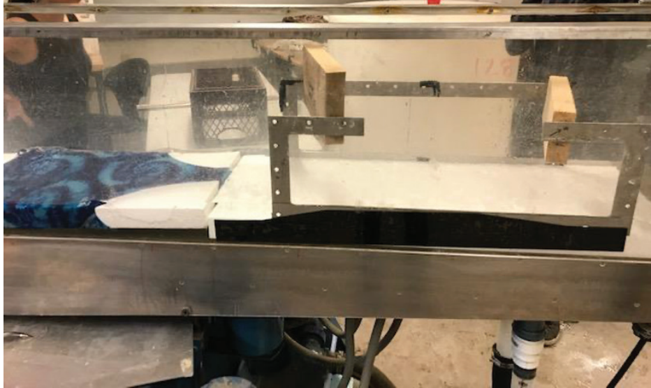
Figure 1. Flume used in the skin friction measurement.
