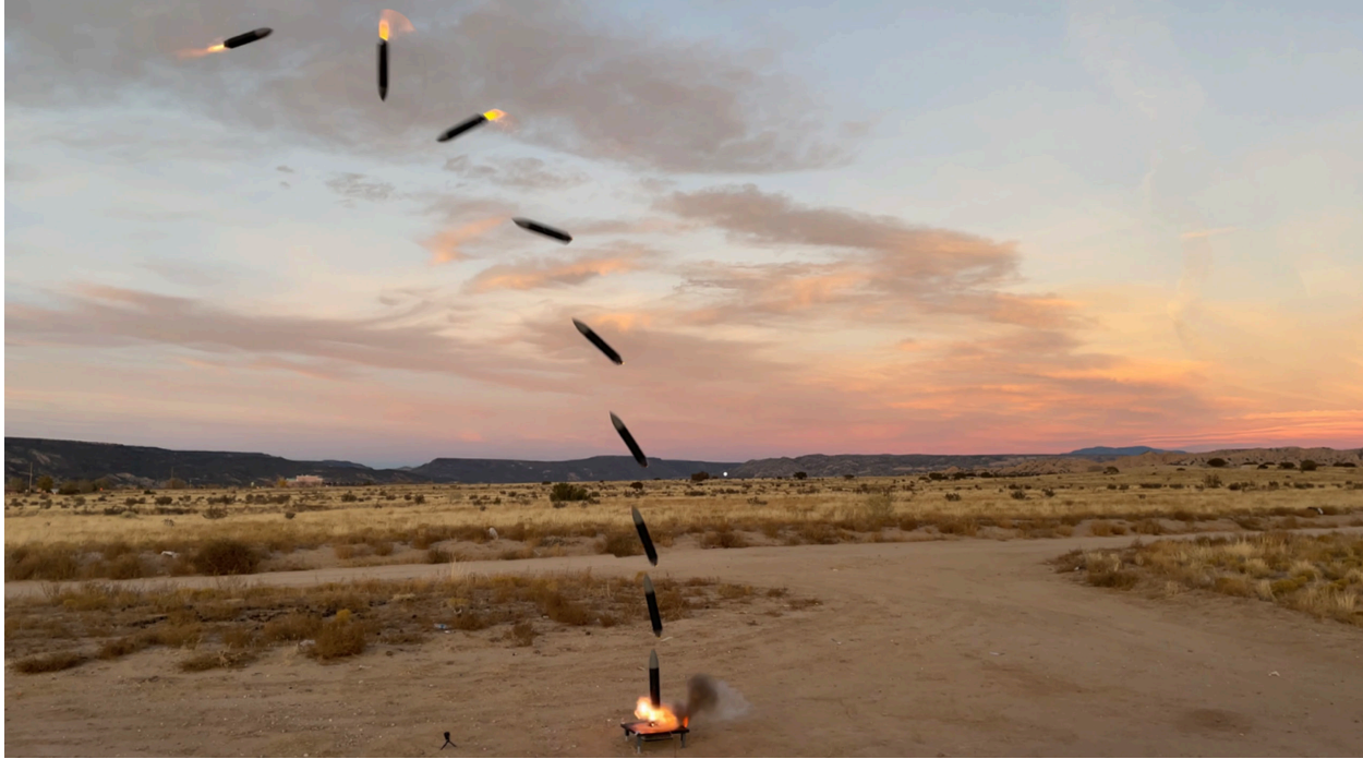
Figure 11. Different phases of the rocket flight are depicted in one photo. By the second and third freeze frames, the abort sequence had already fired, and the rocket was uncontrolled.
