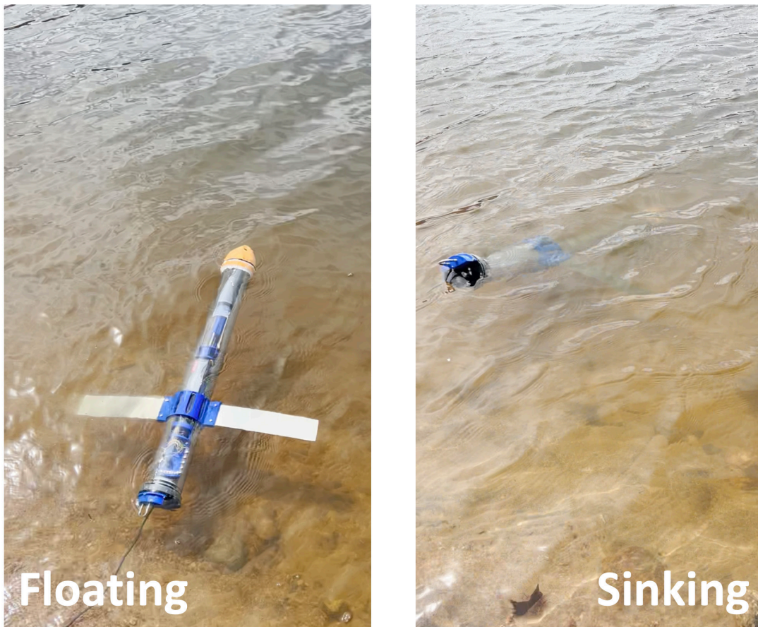
Figure 3: Field test of the AUV's ballast system.
